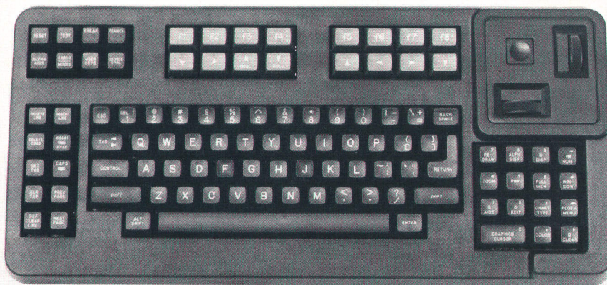
Fig. 2. The HP 2700's keyboard graphics input device consists of two thumbwheels and a button. The thumbwheels are connected to digital shaft encoders.
